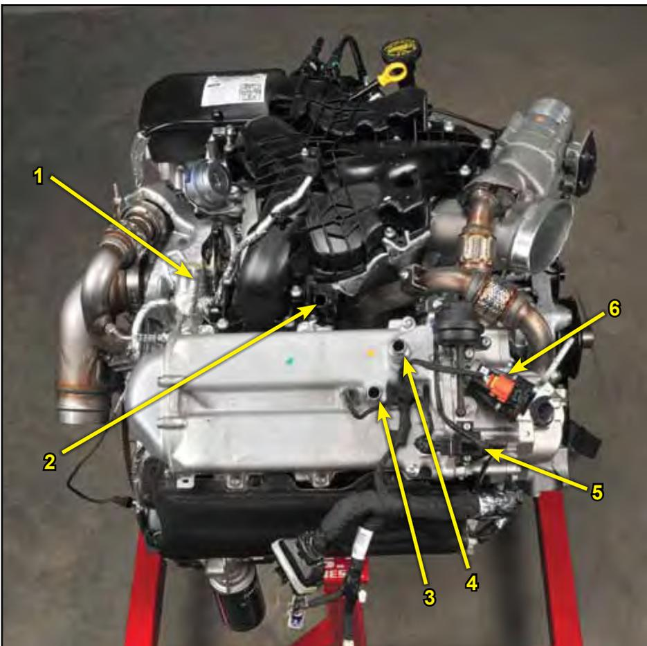
1. Exhaust Pressure (EP) sensor
