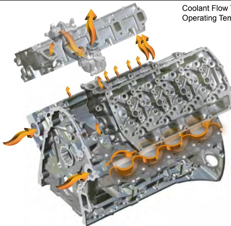
Coolant Flow Through the Block at Operating Temperature (Thermostat Open)
