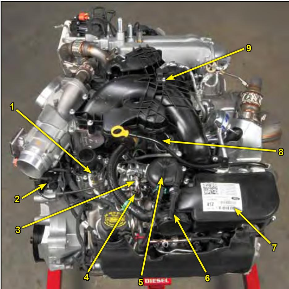
1. Engine Coolant Temperature (ECT) sensor
