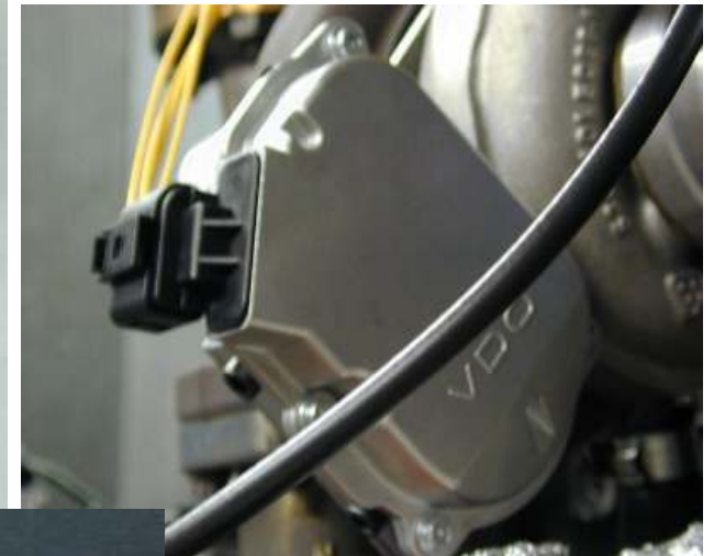
Medium-Torque Electronic Actuator for Intermediate Sized VTG Turbos
